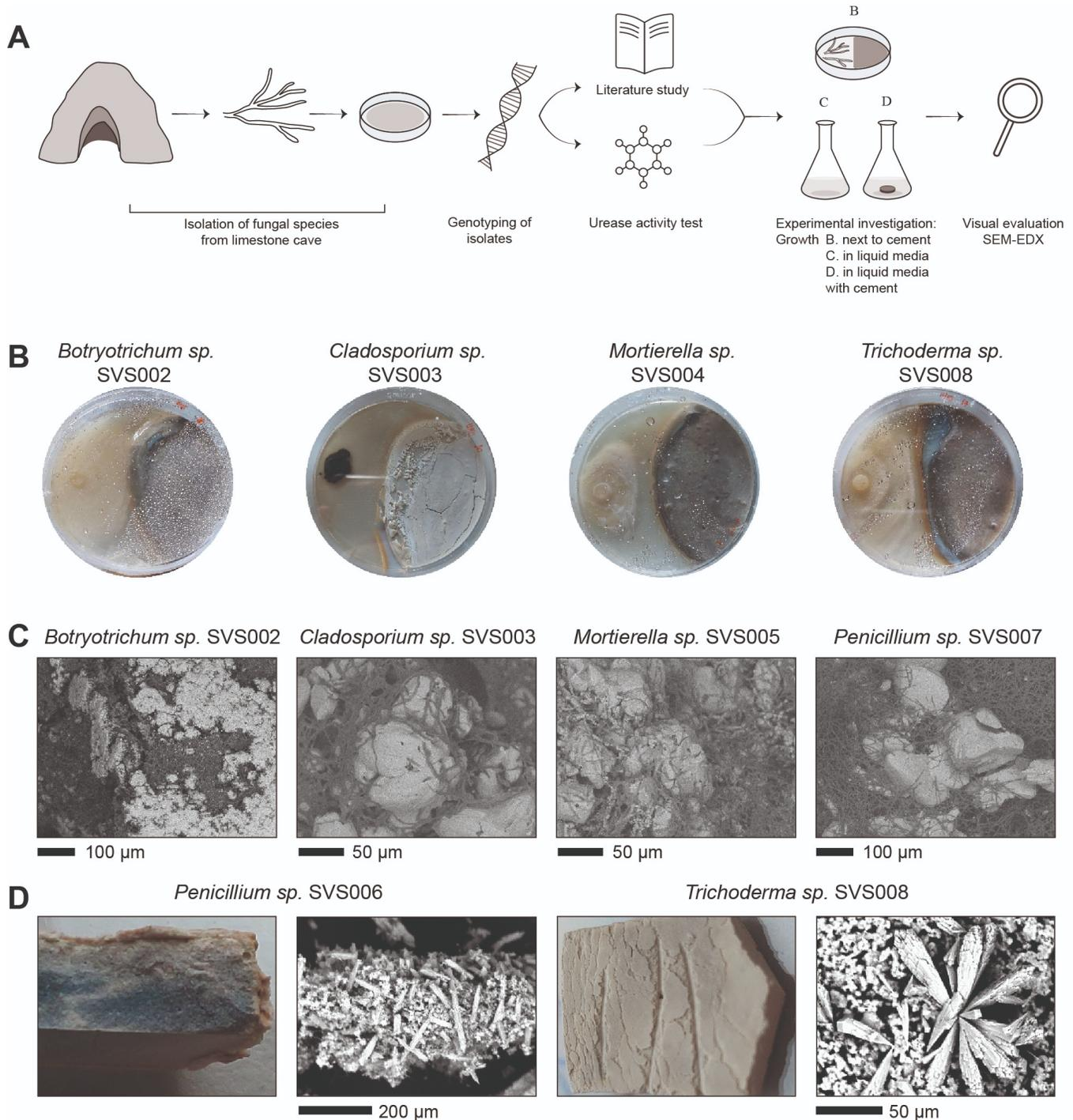
**Figure 1. Screening limestone cave fungi as potential candidates for self-healing concrete: graphical abstract and experimental results:**
